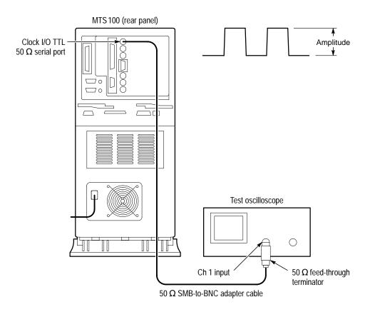
Figure 4–12: Setup for measuring TTL 50 ohm clock pulse amplitude
