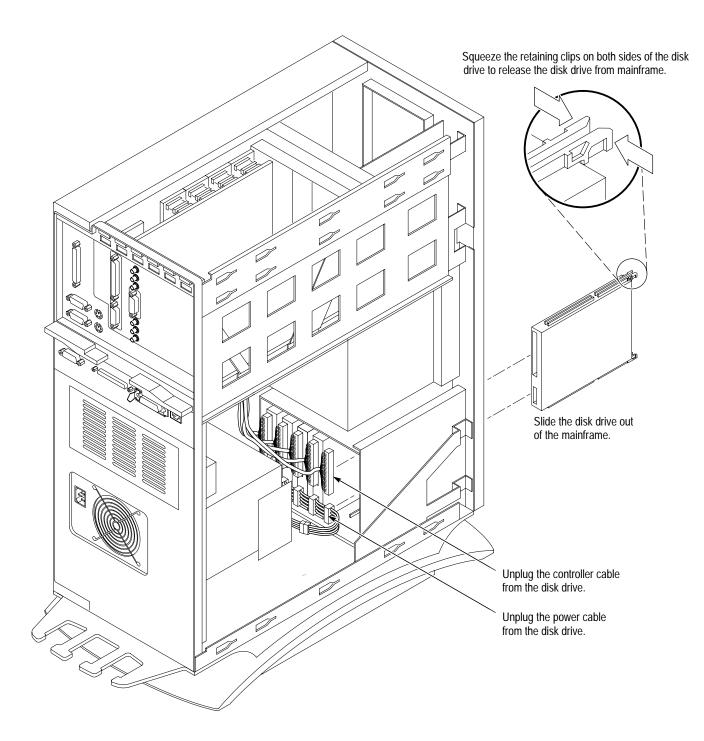
Figure 6–5: Removing Data Store hard disk drives
