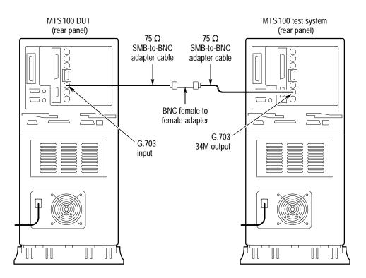
Figure 4-9: Setup for testing G.703 34.368 Mbits/s slave acquisition
