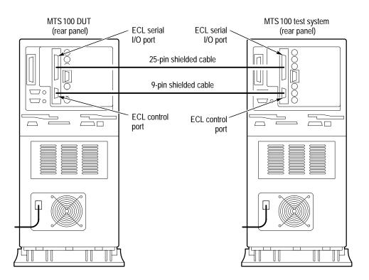
Figure 4–31: Setup for checking ECL serial port slave generation
