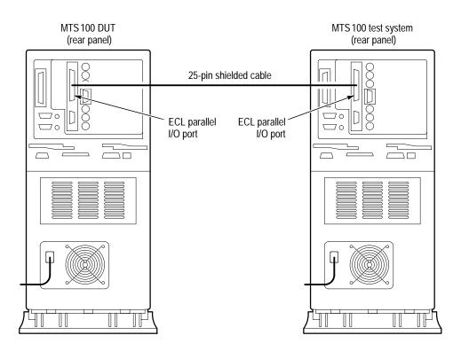
Figure 4–22: Setup for checking ECL parallel port data transfer
