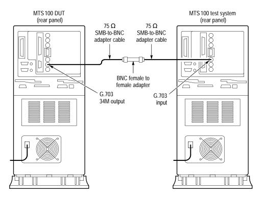
Figure 4–11: Setup for testing G.703 34.368 Mbits/s master generation
