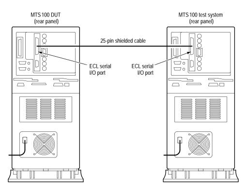
Figure 4–27: Setup for checking ECL serial port slave acquisition and master generation
