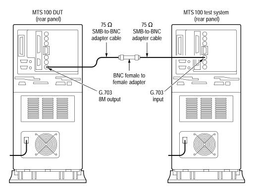
Figure 4-6: Setup for testing G.703 8.448 Mbits/s master generation
