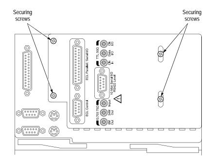
Figure 6–2: MTS 100 rear panel securing screws
