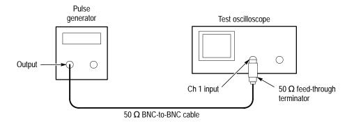
Figure 4-20: Setup for measuring the pulse generator output
