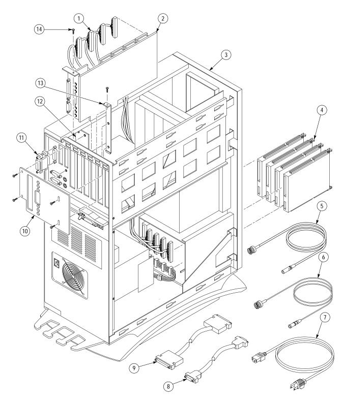
Figure 8–1: MTS100 MPEG Test System
