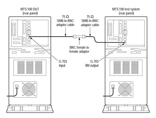
Figure 4-4: Setup for testing G.703 8.448 Mbits/s slave acquisition
