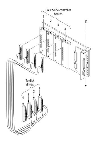
Figure 5–2: Removing the Data Store circuit board
