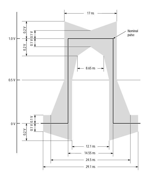
Figure 1–3: Pulse specification for G.703 34.368 MHz
