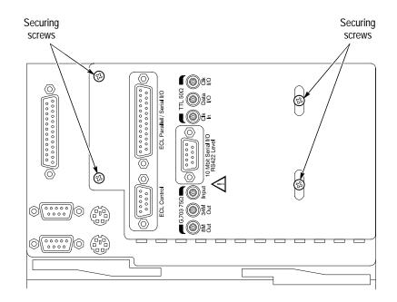
Figure 5–1: Rear panel securing screws.
