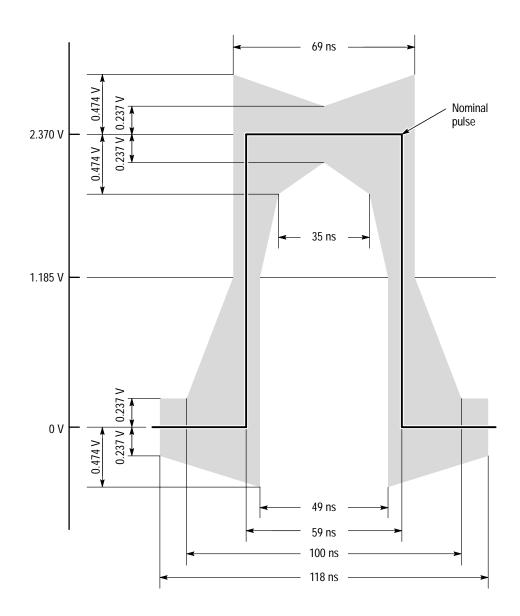
Figure 1–2: Pulse specification for a G.703 8.448 MHz pulse
