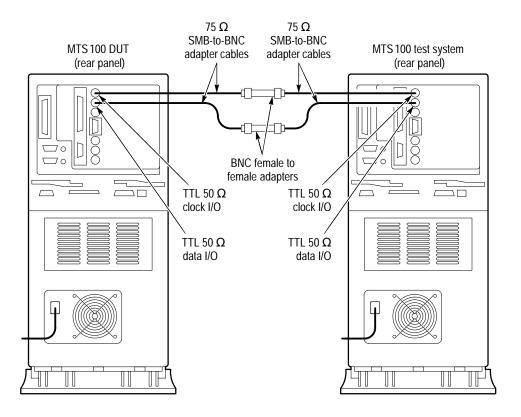
Figure 4–13: TTL 50 ohm slave acquisition and master generation setup
