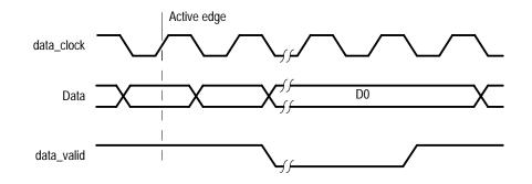
Figure 1–4: Timing diagram for the ECL serial port
