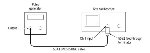
Figure 4–24: Setup for measuring the pulse generator output
