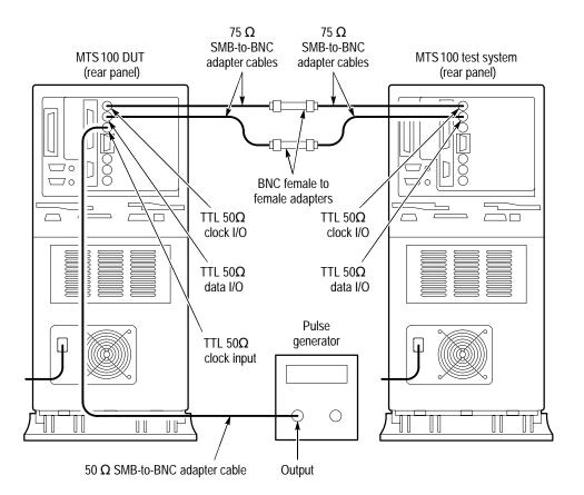
Figure 4–17: Setup for checking 50 ohm external clock generation
