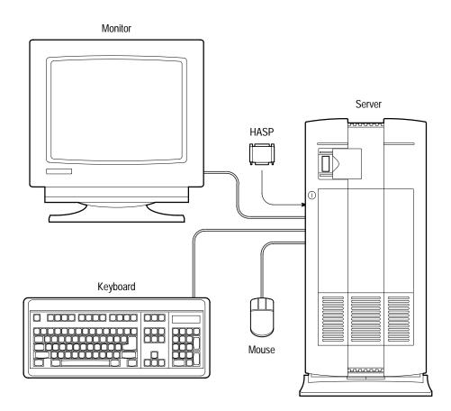
Figure 1–1: Components of the MTS 100 MPEG Test System
