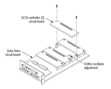
Figure 5–3: Location of the 8.448 MHz oscillator adjustment
