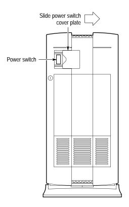
Figure 2-5: Turning on the MTS 100 MPEG Test System
