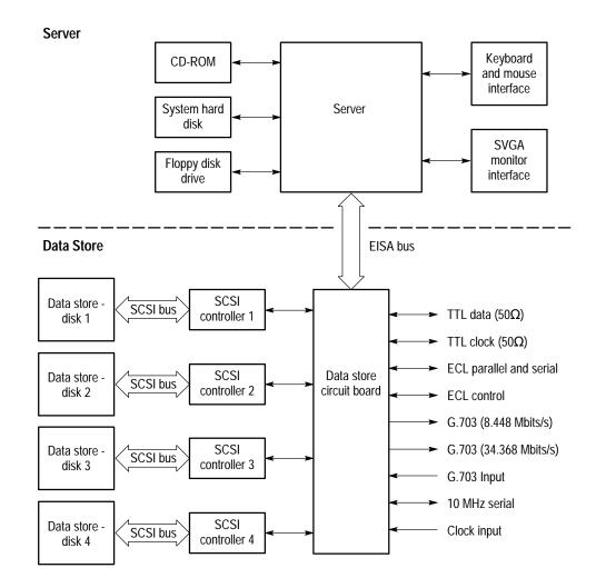
Figure 3–1: Test System block diagram
