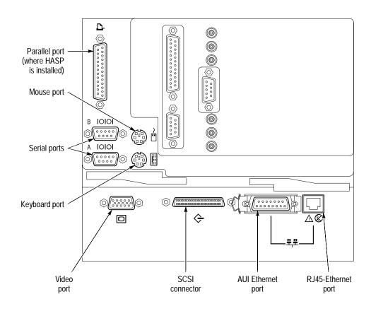
Figure 2–2: The rear panel of the MTS 100 server
