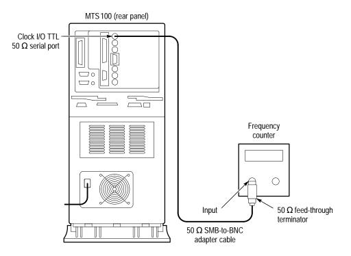
Figure 4–2: Setup for measuring internal clock output accuracy
