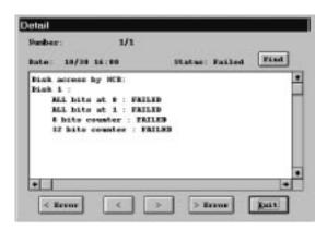
Figure 6–24: Disk access by NCR failure
