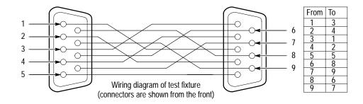
Figure 4–18: 10 MHz signal interconnect fixture
