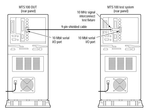
Figure 4–19: Setup for checking 10 Mbit serial port high speed clock slave acquisition and master generation
