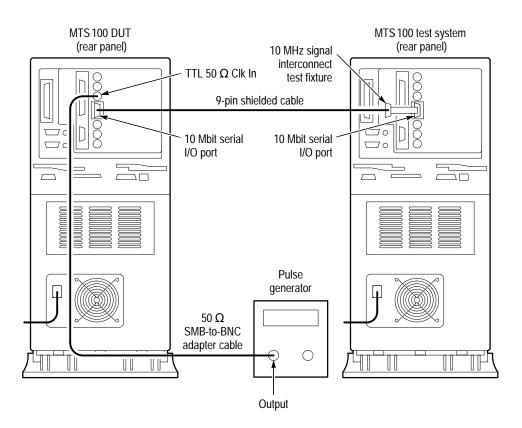
Figure 4–21: Setup for checking 10 Mbit external clock generation
