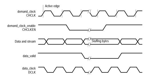
Figure 1–5: ECL Timing diagram with control port
