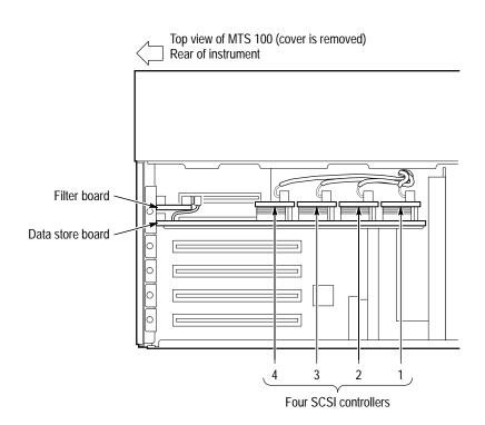
Figure 6–1: Top view of the server
