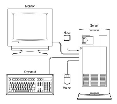
Figure 2–1: The MTS 100 MPEG Test System
